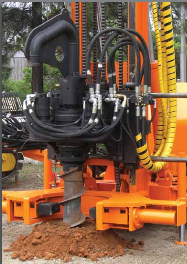
Perfuração com hollow auger - Drilling with hollow auger
